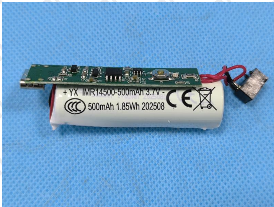
Internal view of battery
